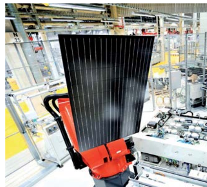
Fully-automated production in our module assembly line in Bitterfeld-Wolfen, Germany
